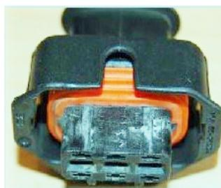
This plug should be as clean as a whistle, and this one is not the worst we've seen. Usually the seal has a greenish deposit on it and the contacts can be seen to be corroded.
